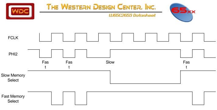
Figure 1-15 System Speed Change Timing Diagram
