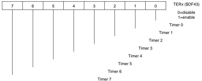
Figure 1-4 Timer Enable Register (TER)
