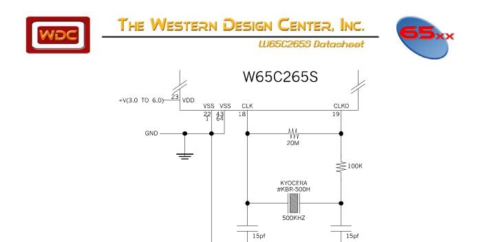
Figure 4-10 W65C265S Resonator Circuit
