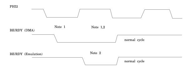
Figure 2-5 BE Timing Relative to PHI2
