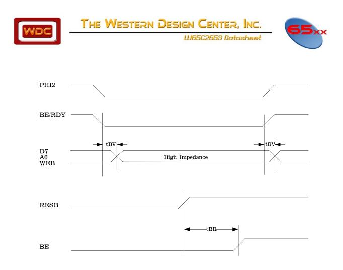
Figure 3-3 AC Timing Diagram #3
