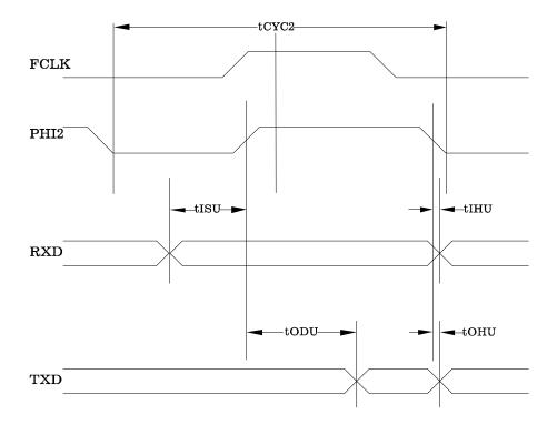
Figure 3-4 AC Timing Diagram #4
