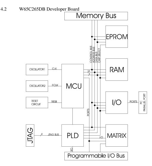
Figure 5-7 W65C265DB Developer Board
