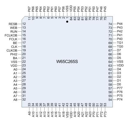
Figure 2-2 W65C265S 84 Lead Chip Carrier Pinout
