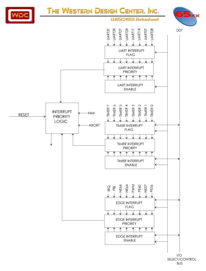
Figure 4-2 W65C265S Interrupt Controller Block Diagram
