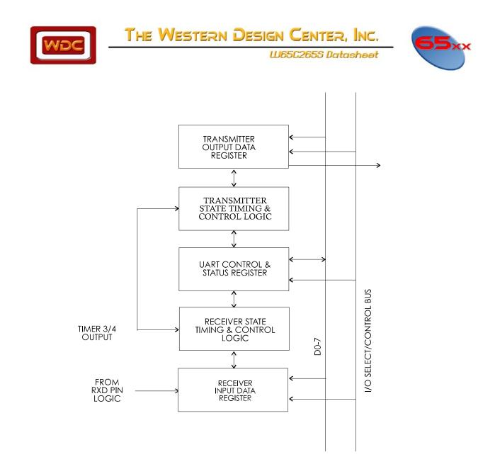
Figure 4-4 W65C265S UART Block Diagram
