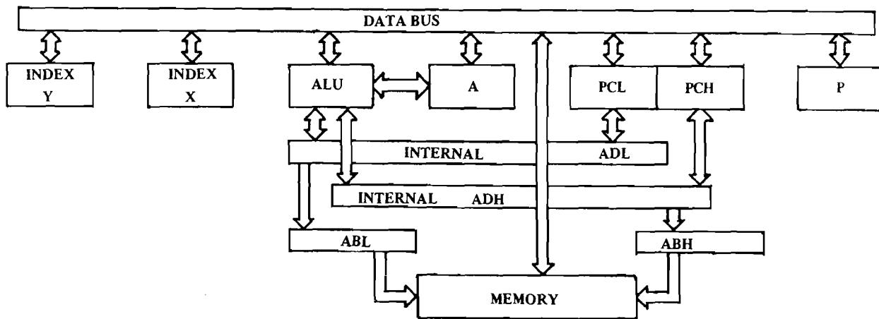
*Partial Block Diagram of MCS650X Including Index Registers*
