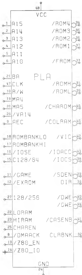
Figure 16-8. The C128 PLA Chip
